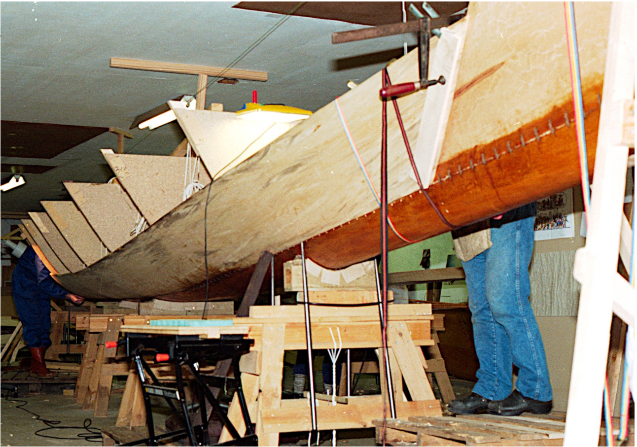
Fig. 5: The Keel Plank, the Middle Plank, the Stem Part and the Keel Horn Assembly.
