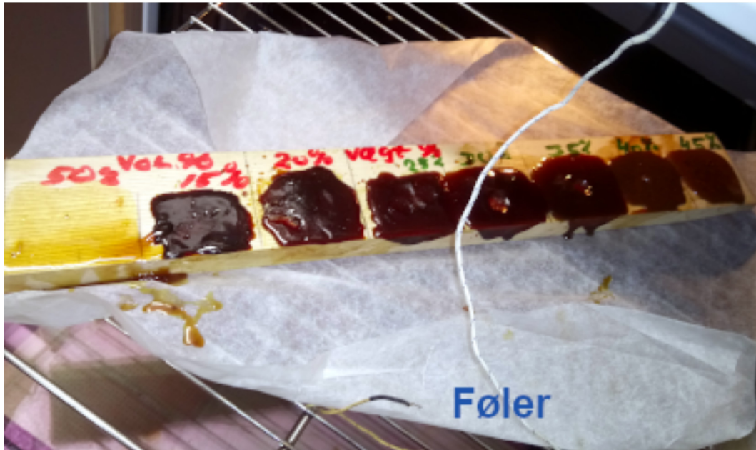
Fig. 3: Testemne for blandingsforhold.
